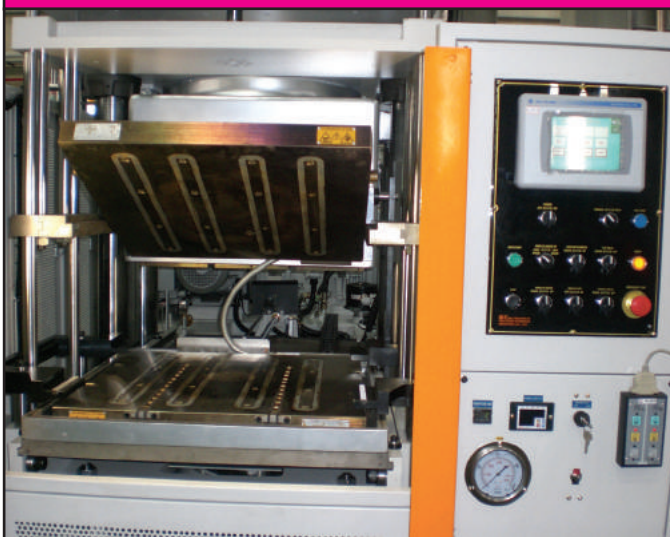
Figure 6 - vertical press with vacuum with magnetic plates and integrated rollers — hand-held control pendant is shown below the main control panel
