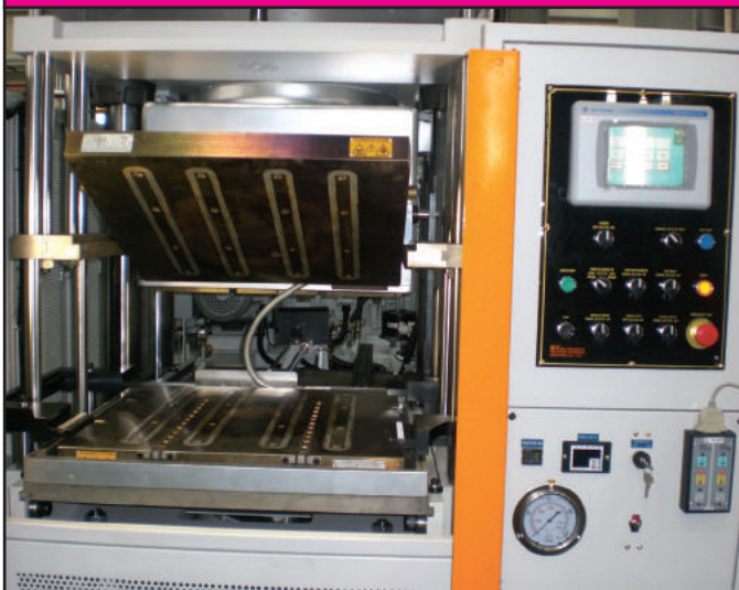
Figure 6 - vertical press with vacuum with magnetic plates and integrated rollers — hand-held control pendant is shown below the main control panel
