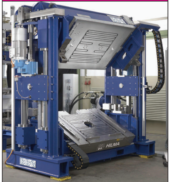
Figure 5 - vertical press with magnetic platens, lower platen has custom mold rollers and guides
